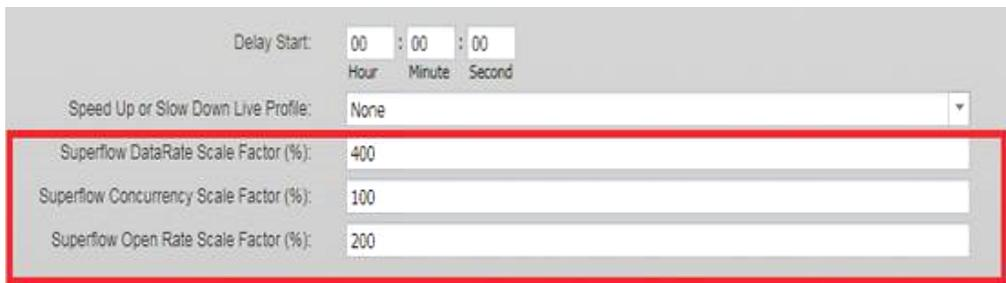
**Note:** The result of these settings are displayed in the LiveAppsim tab of Real Time Statistics and in Report as **Desired data rate**. The Desired data rate is expressed as a percentage (%) of Original data rate.
